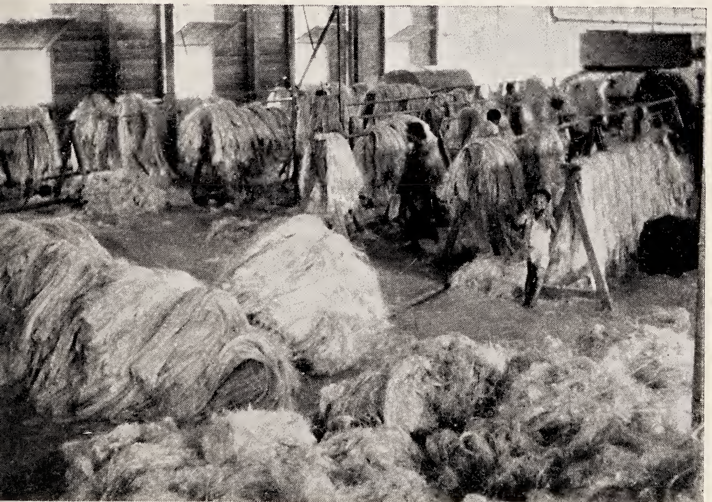
(Central Office of Information) Brushing and grading the stripped hemp.
